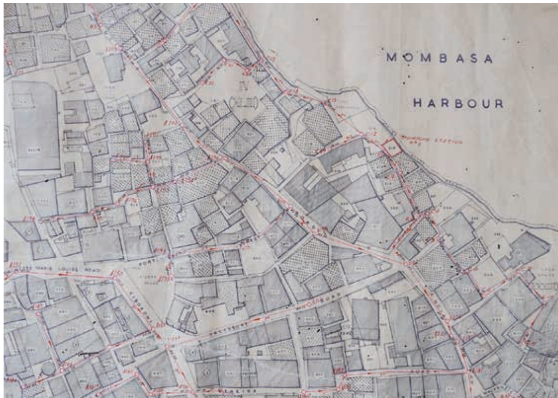
Detail of one of the original planning maps for Mombasa's sanitation system. The plan shows the location of houses, between which are red lines, marking the course of the new sewage pipes and their direction of flow.
